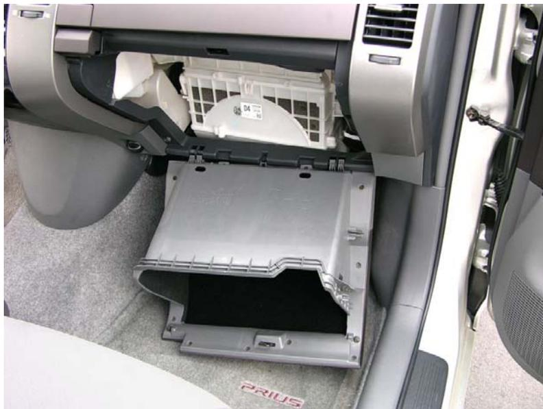
The air-flow assembling will then be completely visible and very easy to access. You'll see the filter at the top, lying horizontal along the entire width of that white plastic air-duct. Just pull on both sides to slide it out. Then you can easily inspect it and replace it (when needed).
