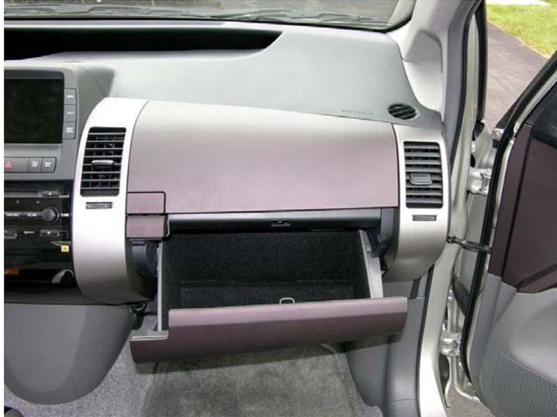
Open the bottom glove-box, then remove all the contents (since they will end up falling out all over the floor otherwise).
