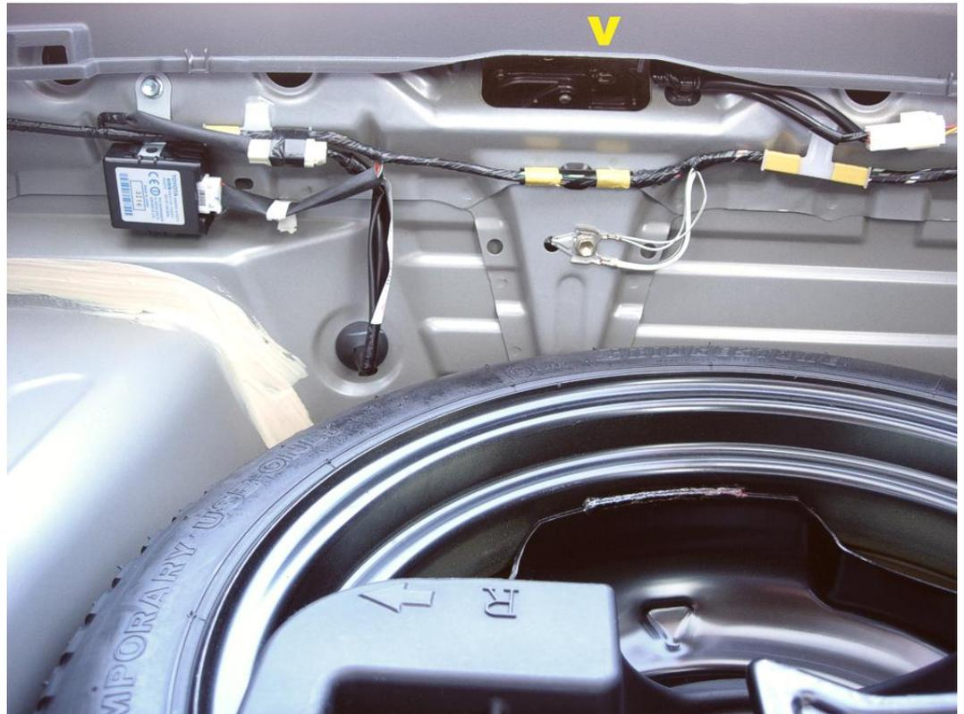
This close-up of the photo above makes the (brass colored) release latch easier to see.
